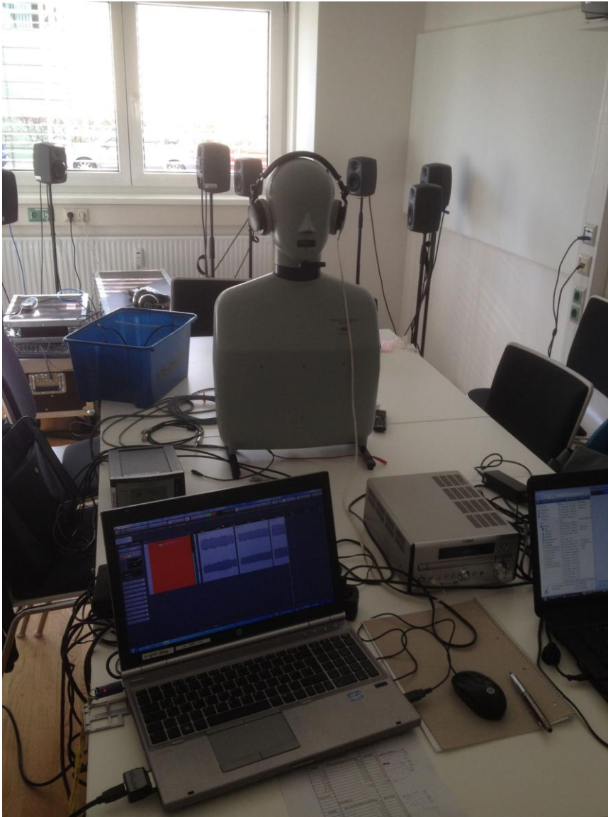
Fig. 11: shows the head simulator and the reconstructed testing situation
