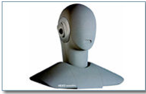
Figure 4.1.1: HEAD acoustics HEAD-Shoulder-Unit III
