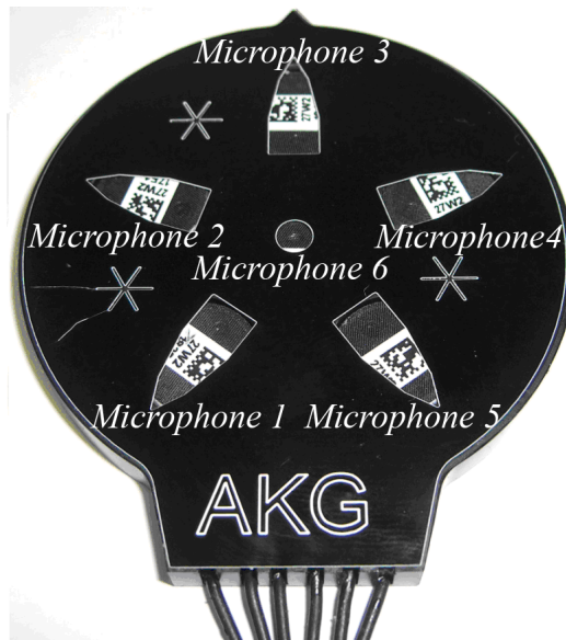
Figure 3.1: Prototype of a second-order circular microphone array.
