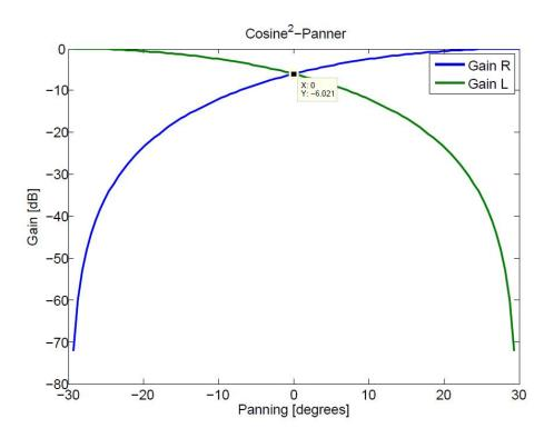
Figure 44: Gain factors of a  $Cosine^2 - Panner$
