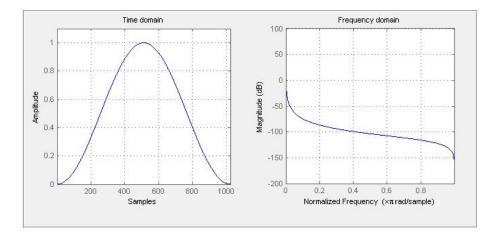
Figure 13: Hann-Window, 1024 samples, time-domain versus frequency-domain
