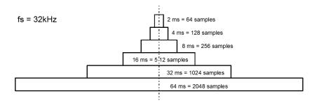
Figure 8: Staged blocklengths for time-domain to frequency-domain transformation
