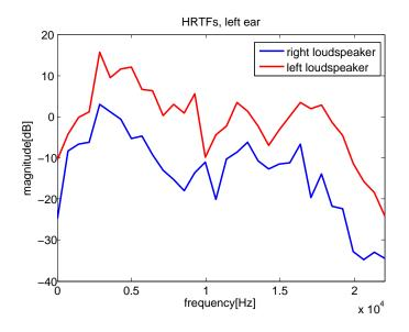
Figure 3: Measured HRTFs, left ear, IR 64 samples
