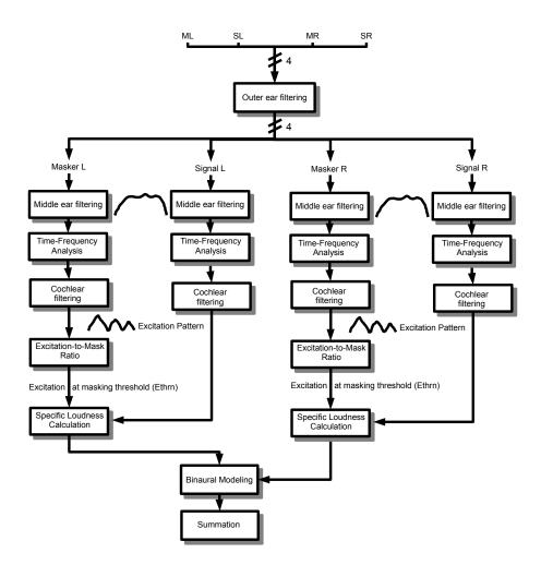
Figure 1: Block diagram of the used hearing model, the inputs SL, ML, SR and MR are signals and maskers of the left and right loudspeaker of the stereo arrangement and will further be explained in section 2.2.1
