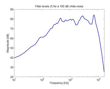
Figure 19: Nonlinear filter bank: filter levels over frequency for a 100 dB white noise
