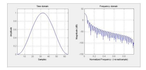
Figure 12: Hann-Window, 64 samples, time-domain versus frequency-domain
