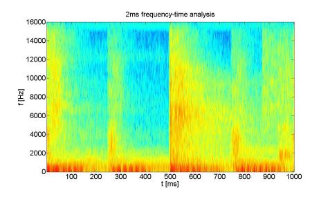
**Figure 9:** Spectrogram, blocklength = 2 ms
