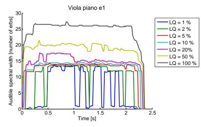
Figure 56: Spectral width for an unmasked sample of a viola, playing a piano e1, different LQs
