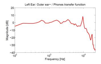
Figure 6: Measured outer ear- / phones transfer function, left ear
