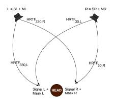
Figure 2: Crosstalk schematic for stereo setup
