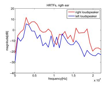
Figure 4: Measured HRTF, right ear, IR 64 samples
