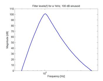
Figure 18: Nonlinear filter bank: filter levels over frequency for a 1kHz, 100 dB sinusoid
