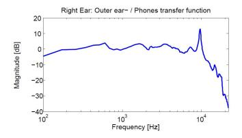
Figure 5: Measured outer ear- / phones transfer function, right ear
