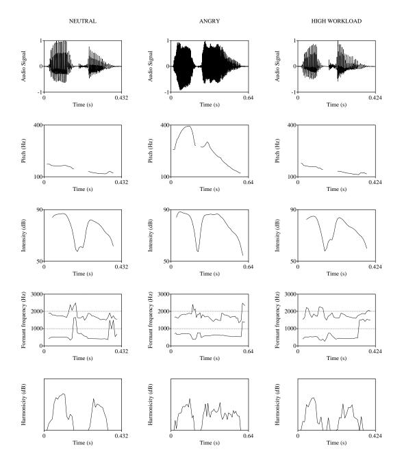
**Figure 3.14.:** PCM waveforms and a variety of extracted features for the word *enter* (from the SUSAS database) spoken under three different stress conditions.
