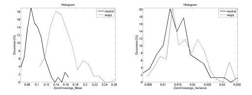
Figure 3.13.: Histogram plots of zero-crossing rates for talking styles angry vs. neutral (Emo-DB database)
