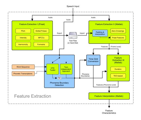
Figure 4.1.: Flow chart of the feature extraction stage.
