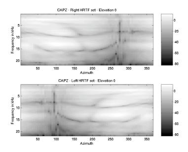
**Figure 4.4** Modelled KEMAR set from 0°-360° azimuth/0° elevation as a function of time and frequency
