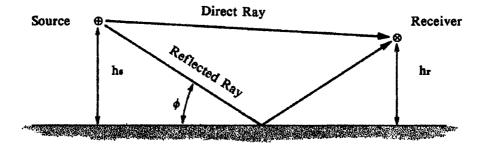
Figure 3.8 Geometry for reflection of sound from level ground of finite impedance.
