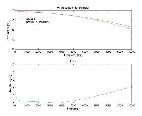
Figure 3.4 Desired frequency response and actual frequency response designed with a Yulewalker recursive IIR filter
