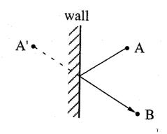
Figure 3.12 Single wall reflection and corresponding image source A'
