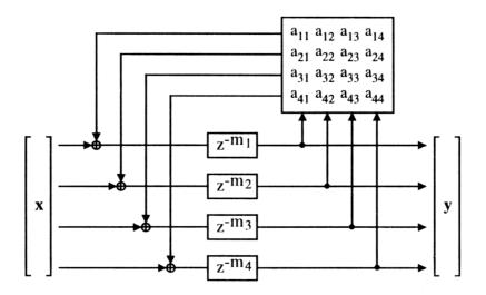
Figure 3.23 Stautner and Puckette's four-channel feedback delay network [3]
