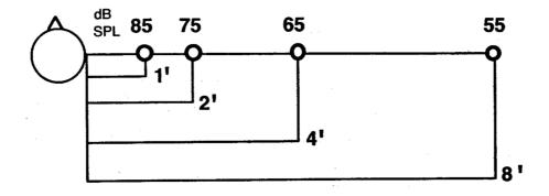
Figure 1.21 Reduction of intensity using loudness scales based on sones [1]
