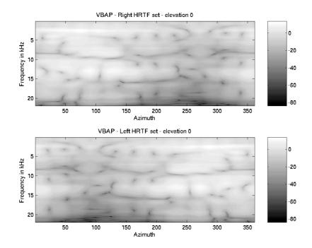
**Figure 4.13** 360 VBAP - interpolated HRTFs (0° - 359° azimuth, 0° elevation) as a function of time and frequency, using a 30° raster of azimuth and elevation
