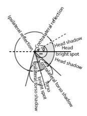
Figure 1.14 The Snowman model and The Torso-Shadow Cone [6]
