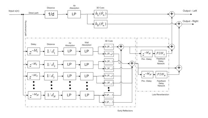
Figure 5.1 The Signal Routing of the 3D System
