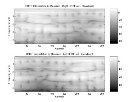
**Figure 4.16** Residue interpolated HRTF set (azimuth 0° - 359°, elevation 0°) as a function of time and frequency - 30° raster -
