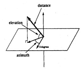
Figure 1.4 Azimuth, elevation and distance in the vertical polar system [1]
