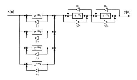
Figure 3.21 Schroeder's reverberator consisting of a parallel comb filter and a series allpass filters [3]
