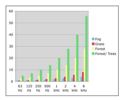
Figure 3.10 Diagram of different absorption coefficients of different environments
