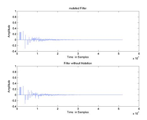
Figure 3.26 Impulse Response of the permuted FDN and the original FDN of Jot
