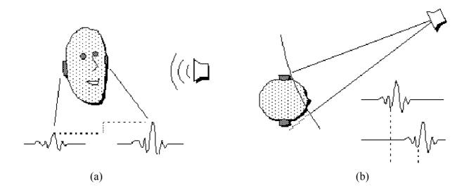
Figure 1.10 A simple method for deriving IID (a) and ITD (b) [Internet]
