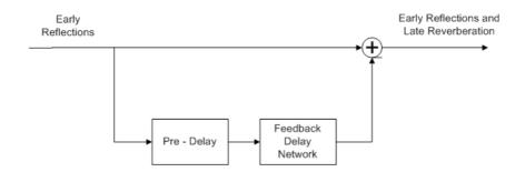
Figure 3.27 Simplified signal flow of the system
