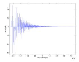
Figure 3.22 Impulse response of the Late Reverberation Filter of Schroeder
