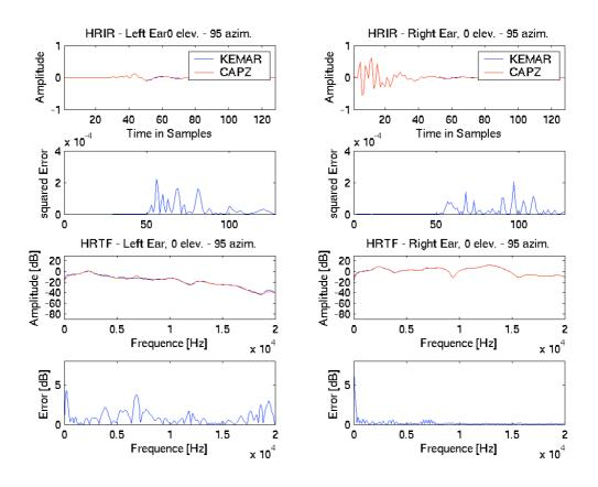
Figure 4.5 CAPZ Model compared to the desired Kemar curve of 95° azimuth/0° elevation - with 50 zeros –
