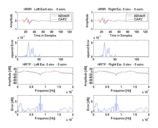
Figure 4.2 CAPZ Model compared to the desired Kemar curve of 0°azimuth/0°elevation - with 40 zeros -
