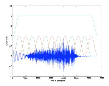
Figure 5.3 Block filter technique using hanning windows
