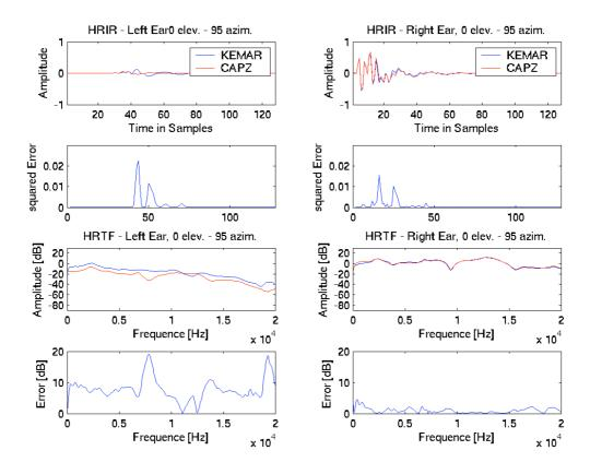
Figure 4.3 CAPZ Model compared to the desired Kemar curve of 95° azimuth/0° elevation - with 40 zeros -
