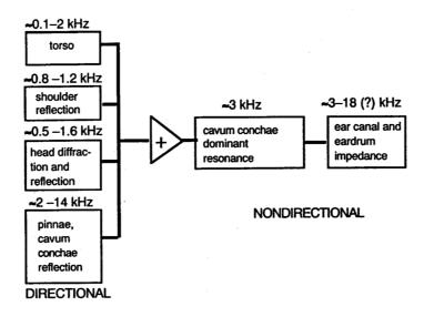
Figure 2.1 Directional and nondirectional components of the HRTF [1]
