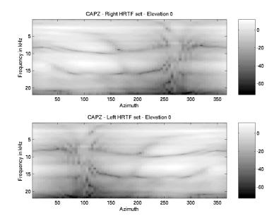
**Figure 4.9** CAPZ HRTF set (0° - 355° azimuth, 0° elevation) as a function of time and frequency
