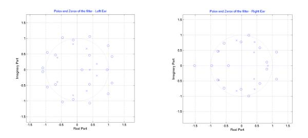
Figure 4.7 Poles and zeros of a CAPZ model, left and right ear (0° azimuth, 0° elevation)
