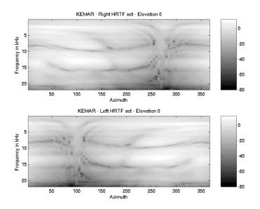
**Figure 4.8** Kemar HRTF set (0° - 355° azimuth, 0° elevation)
