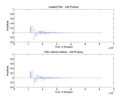
Figure 3.29 Pre-delayed impulse response of the original and the permuted FDN
