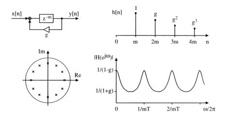
Figure 3.19 Comb filter: flow diagram, time response, frequency response, and pole diagram (clockwise from top-left) [3]
