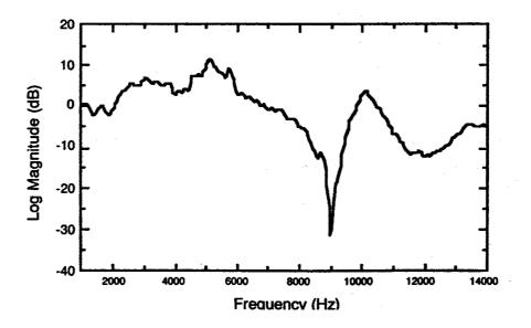
Figure 2.7 Difference in spectra between two front-back source locations on a cone of confusion: 60 and 180 degrees azimuth, 0 degrees elevation. [1]
