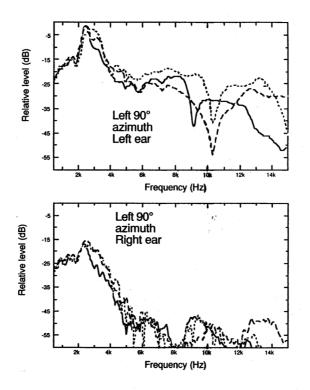
**Figure 2.4** HRTFs of left and right ear, 90° azimuth and 0° elevation, measured for three people [1]
