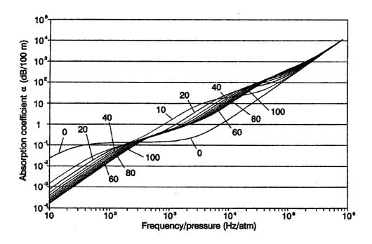
**Figure 3.2** Sound absorption coefficient in air (dB/100 m) versus frequency/pressure ratio for various relative humidity at 20°C. [15]
