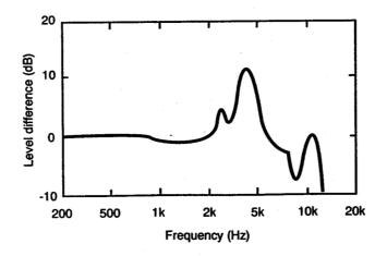
Figure 2.2 Ear canal resonance [1]
