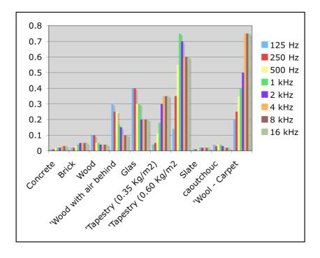
Figure 3.6 Table of different absorption coefficients for different wall, roof and floor materials
