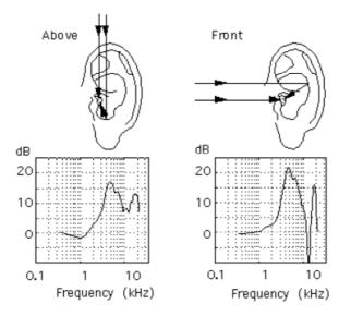
Figure 1.13 Frequency responses of the pinna for two directions of arrival [1]
