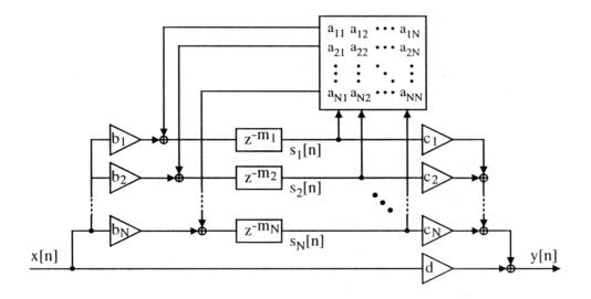
Figure 3.24 Feedback delay network as a general specification of a reverberator containing N delays [3]
