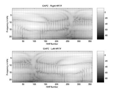
**Figure 4.12** 360 VBAP - interpolated HRTFs (0° - 359° azimuth, 0° elevation) as a function of time and frequency, using a 10° raster of azimuth and elevation
