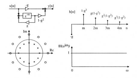
**Figure 3.20** Allpass filter formed by modification of a comb filter: flow diagram, time response, frequency response, and pole-zero diagrams (clockwise from top-left) [3]
