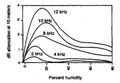
Figure 1.22 AIR Absorption [1]
