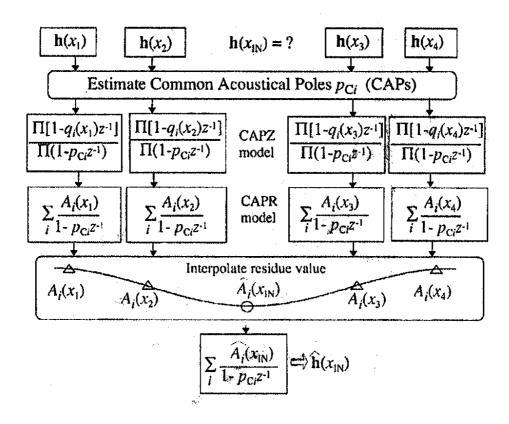
Figure 4.14 The Common Acoustical Pole and Residue interpolation method [18]
