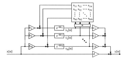
Figure 3.25 Feedback delay network as a general specification of a reverberator containing N delays and a permutation matrix M
