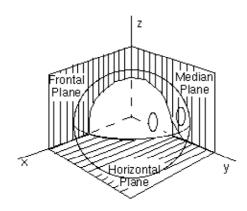
Figure 1.2 Head-centered rectangularcoordinate system [20]
