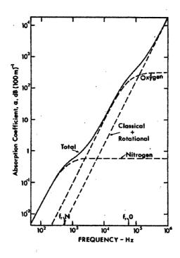
**Figure 3.1** Predicted atmospheric absorption in dB/100m for a pressure of 1 atm, temperature of 20°C and relative humidity of 70 % [15]
