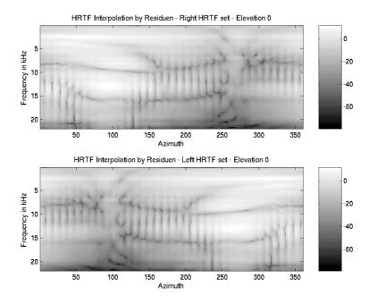
Figure 4.15 Residue interpolated HRTF set (azimuth 0°- 359°, elevation 0°) as a function of time and frequency - 10° raster -
