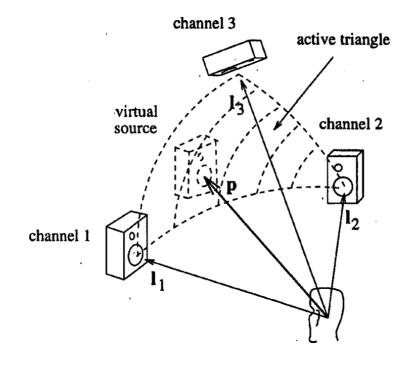
Figure 4.10 The region on the surface of the sphere – The active triangle
