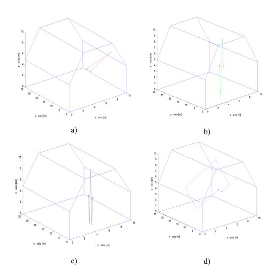
**Figure 3.15** Examples of first a), second b), third c) and fourth 4) order reflections for a simple room.
