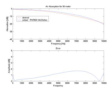
Figure 3.3 Desired frequency response and actual frequency response designed with the Parks-McClellan optimal equiripple FIR filter
