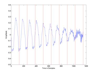
Figure 5.2 Input signal is divided into blocks of the length of 128
