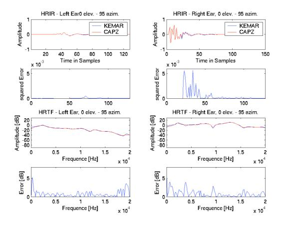
Figure 4.6 CAPZ Model compared to the desired Kemar curve of 95° azimuth/0° elevation - with 20 zeros and zeropadding -
