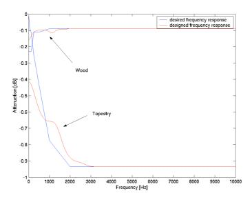
Figure 3.7 Frequency responses of different wall absorption filters
